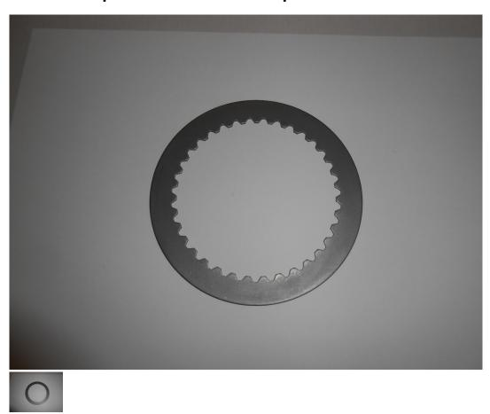
Steel clutch plate for all Maico models 1983 up till today. 6 pieces are needed together with a mixed sinter and organic system. For a cpl. organic system you have to use 5 pieces. A full sintered 6 spring clutch system needs 7 pieces!
